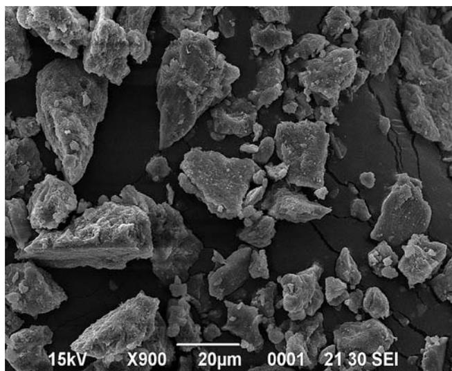
**Fig. 3.** Electron micrograph of clinoptilolite crystals, Magnification  $\times 900$ .
