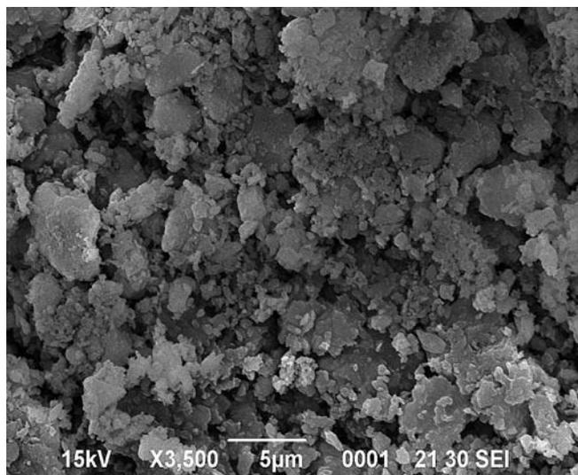
**Fig. 6.** Electron micrograph of clinoptilolite crystals, Magnification  $\times 3500$ .
