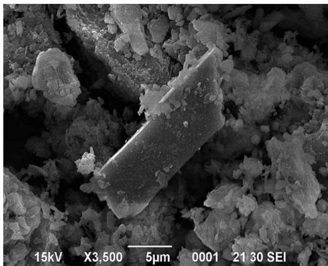
**Fig. 4.** Electron micrograph of clinoptilolite crystals, Magnification  $\times 3500$ .
