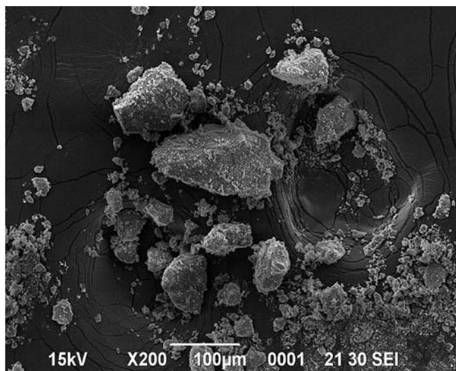
**Fig. 1.** Electron micrograph of clinoptilolite crystals, Magnification  $\times 200$ .
