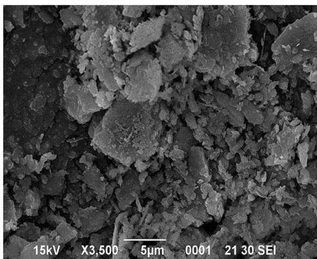
**Fig. 5.** Electron micrograph of clinoptilolite crystals, Magnification  $\times 3500$ .
