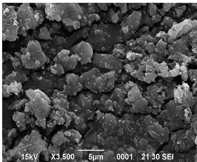
**Fig. 7.** Electron micrograph of clinoptilolite crystals, Magnification  $\times 3500$ .
