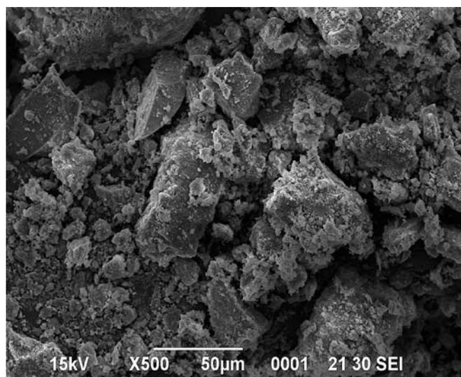
**Fig. 2.** Electron micrograph of clinoptilolite crystals, Magnification  $\times 500$ .
